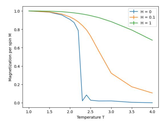
**Question C.2.** For this question, we set T = 1, and we perform 100 runs each for each of the external fields H = 0.1 and H = 1. For H = 0.1, after 98 of the 100 runs, the spins were aligned on the same direction with the external field (positive magnetization). For H = 1, all 100 runs led to a positive magnetization. Thus, we conclude that indeed the direction oriented along the field is preferred in this case.
