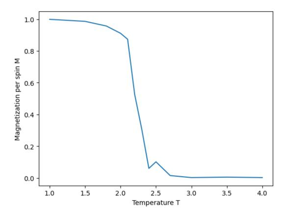
**Question A.3.** We redo the experiment for several values of J. We always focus on a temperature range around 2.2T. The results of our analysis are included in the table below. The analysis shows that the dependence of the transition temperature T on the exchange parameter J is very well described by a line passing through the origin, with slope  $2.29 \pm 0.03$ .
