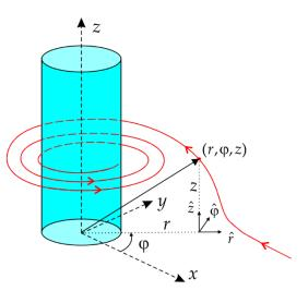
**1.a.** Determine a mathematical expression for the velocity of a fluid particle at a distance r form the axis, in the outer region of the vortex. The fluid particle enters the outer region at a distance  $r_0$  from the axis, with the radial speed  $v_0$ . In the outer **p** region of the vortex the air flow is not rotational.
