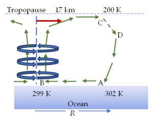
segment A – B is essentially an isothermal process at the temperature  $T_1 \cong 300$  K.
