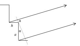
It is obvious that for  $\alpha = 0$ , the path length difference  $\delta$  between two neighboring light rays is (n-1)h. This difference increases with  $\alpha$ .
